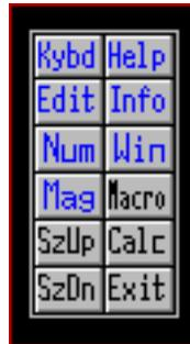
The Control panel allows you to open and close all My-T-Touch panels. Click on each key to perform the toggle action. Blue (highlighted) letters indicate an open panel, black letters indicate a closed panel.
