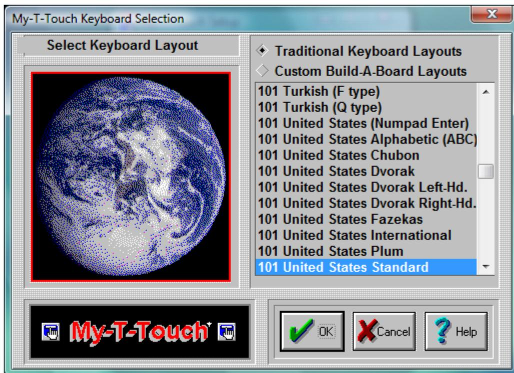
My-T-Touch can operate with many different keyboard layouts. By selecting the same keyboard layout that Windows uses, you can synchronize the display on My-T-Touch with the characters generated in your application.
