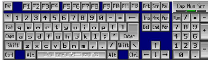
When you click any of the keys on the Keyboard (Alpha) Panel, Edit Panel, and Numeric Panel, they will respond exactly like the corresponding keystroke on a physical keyboard. In order to type with My-T-Touch, another window must be the Active Application and have the input focus. Windows typically indicate where typed characters will be displayed by the Caret, or text cursor. This usually is displayed as a flashing bar, although other shapes may be used.
