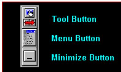
The Tool Button opens and closes My-T-Touch Control Panel in the normal / Supervisor Mode. In Operator Mode, the Tool Button does not function.
