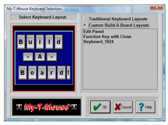
There are a few sample, custom Build-A-Board Layouts available. Additional Build-A-Board layouts can be created, and when placed in the Installation Folder will be added to this list. When selected, the KEYBOARD.KBF in the users configuration folder is replaced with the selected layout. When My-T-Mouse is run, the layout is recognized, and the Build-A-Board compatible run-time (MYTSOFT2.EXE) is used to operate with the version 2.x keyboard layouts.
