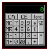
The calculator is a standard four function calculator. To operate simply press the desired number, press an operation key, press the next number, and press an operation key or the total (=) key. You may then send the displayed number to the active window by pressing the SD (Send) button. While there is a number stored in memory, the calculator's display window frame will change color to indicate that memory has a value stored.
